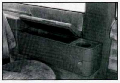
If you have a beverage cooler, lift up on the armrest to open. The cooler has a drain system that drains off as much fluid as necessary. There is also has an ashtray and a cupholder for your convenience.
